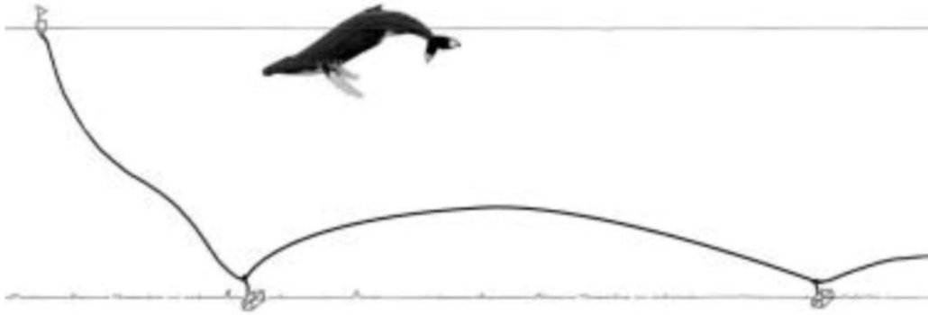
Figure 2. Schematic drawing of a lobster trawl creel in Massachusetts with floating groundline, showing the elevated groundline reaching 16 ft (approx. 5m), vertically suspended leg ropes and the 90 ft (approx. 27 m) distance between traps (from McKiernan et al. (2002))
