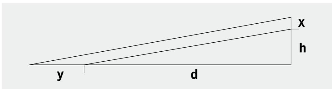
**Figure 1. A relatively small increase (x) in the height (h) of the harpoon as a wave lifts the bow of the ship, results in a large change in projection (y) of a harpoon aimed just before the wave at a whale at a distance (d) from the whaling ship, which would have to be compensated during the wave motion in order to try to maintain the aim (for further explanation see the text).**
